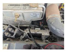
2) Uplug the small connector on the Top Right of the computer. It will have 16 Pins
