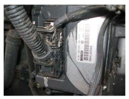
4) Connect the Stock ECM connector to the Male Connector from the module. Note: Make sure to completely push together until the connector clicks.
