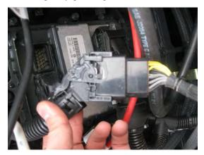
5) Unplug MAP sensor and Plug Female connector from module into the Map Sensor, then connect the Female Map Connector to the Male connector of the module.
