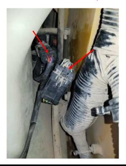
**6)** Route power and ground leads along factory wiring loom to the battery. Connect red wire with ring terminal to positive battery post. Connect the Black wire with ring terminal to negative battery post.
