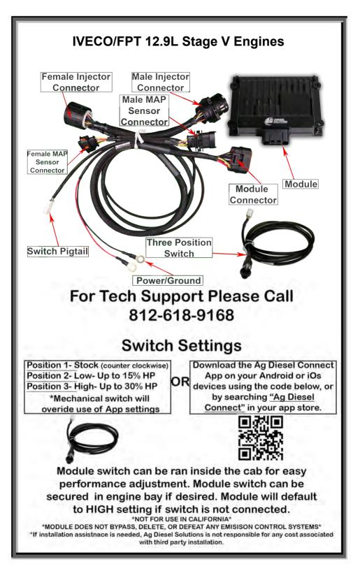
**1)** Locate the injector connector and MAP sensor on the right side of the engine.
