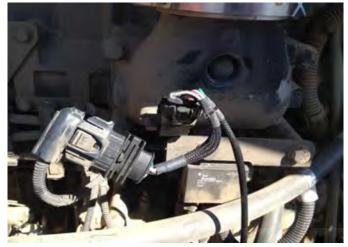
**7)** Connect Red wire with ring terminal to a 12V constant source (i.e. alternator)
