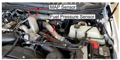
**2)** Unplug the fuel pressure sensor. It is located at the end of the Common Fuel Rail. The Common Fuel Rail runs alongside the valve cover.
