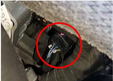
3) Plug male connector from module into fuel pressure sensor. Plug the stock connector to the female connector from the module.
