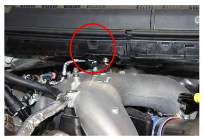
6) Plug the male connector from the Ag Diesel Solutions module into the stock MAP sensor. Then plug the male connector from the module into the stock male MAP sensor connector.
