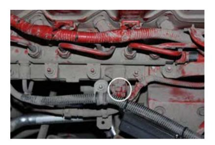
**7)** Plug the Ag Diesel Solutions female MAP sensor connector into the stock male MAP sensor. Plug the Ag Diesel Solutions male MAP sensor connector into the stock female MAP sensor connector.
