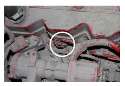
**3)** Route the Module Harness as shown in the picture below. The Module Case will be located closer to the Flywheel side of the engine.
