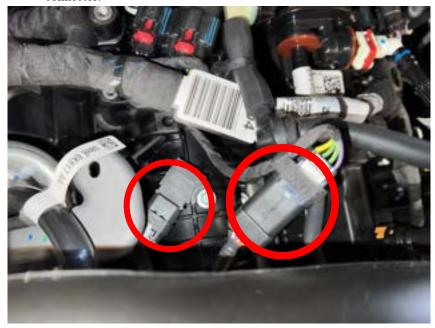
**5)** Disconnect stock T-MAP sensor connector by pulling back on locking tab and squeezing the connector release tab.
