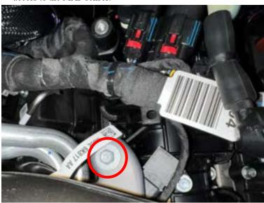
**3)** Disconnect stock MAP sensor connector by pulling back on locking tab and squeezing the connector release tab.
