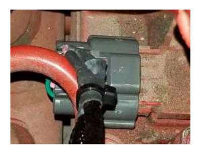
8) Connect the red wire with ring terminal to a +12V constant source, such as the intake air heater grid relay. Connect the black wire with ring terminal to a good Chassis Ground.
