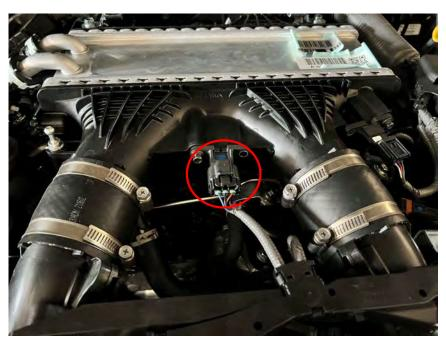
**5**) Connect the ADS female T-MAP connector to the factory T-MAP sensor. Connect the ADS male T-MAP connector to the factory female T-MAP sensor connector.
