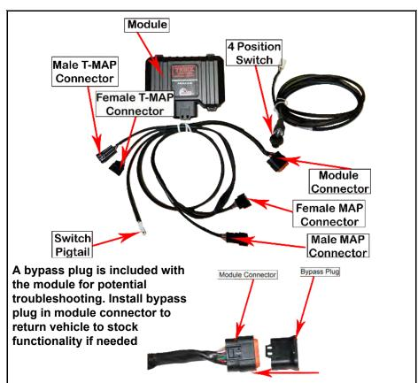
Make sure to push completely together until connector snaps when using bypass plug.
