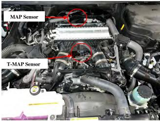
2) Disconnect the factory female MAP sensor connector from the MAP sensor by pressing down on the release tab and pulling out of the sensor.
