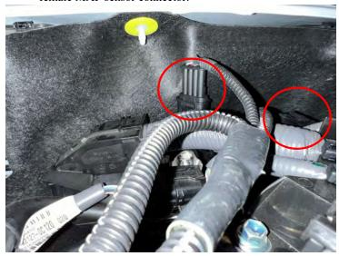
**4)** Disconnect the factory female T-MAP sensor connector from the T-MAP sensor by pressing down on the release tab and pulling out of the sensor.
