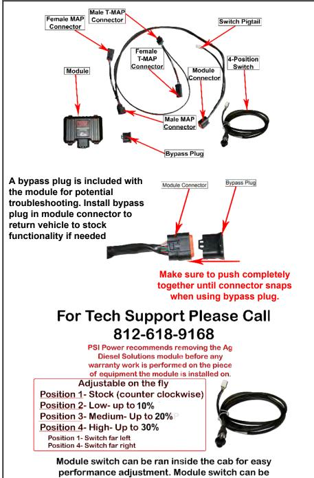
Module switch can be ran inside the cab for easy performance adjustment. Module switch can be secured in engine bay if desired. Module will default to HIGH setting if switch is not connected
