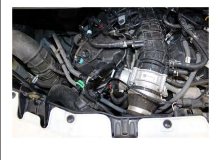
**7)** Remove the bypass plug from the Ag Diesel Solutions harness, and plug the harness into the module.
