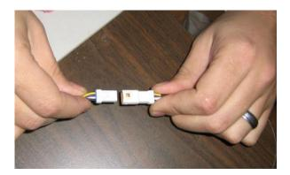
**8)** Remove the bypass plug from the Ag Diesel Solutions harness, and plug the harness into the module.
