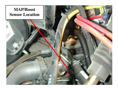
Locate the MAP sensor as shown in the picture above. The image to the right is a close-up view of the stock MAP sensor.
