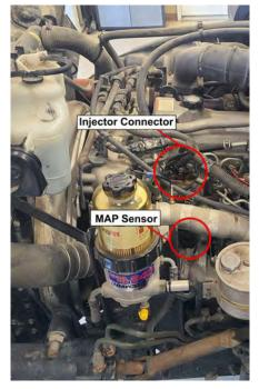
2) Disconnect the stock male injector connector.
