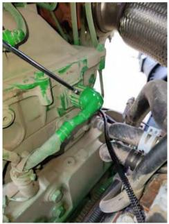
**2)** Connect male module connector into factory female connector in cylinder head. Connect female module connector into male factory harness connector.
