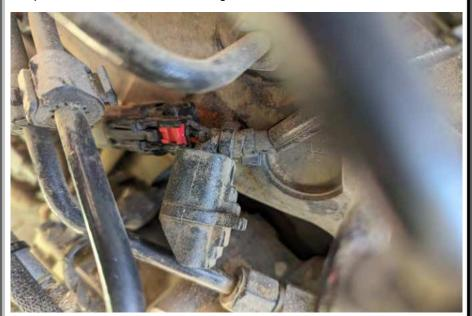
**5)** Connect the module male connector into fuel pressure sensor female pigtail. Connect the module female connector into fuel pressure sensor factory wiring harness male connector.
