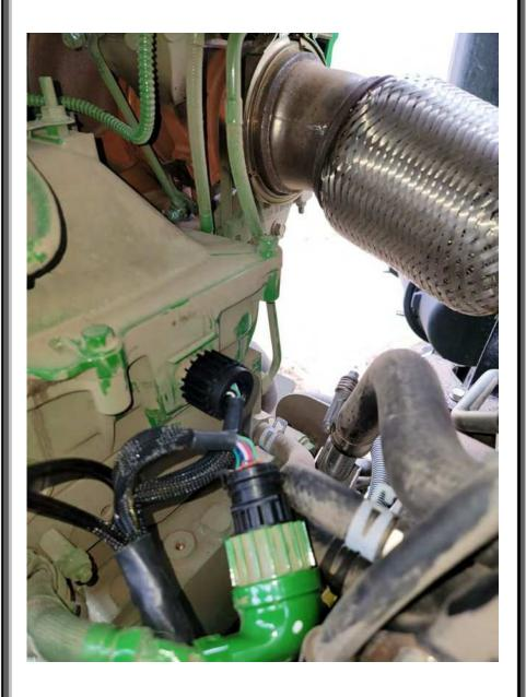
3) Locate fuel pressure sensor pigtail.
