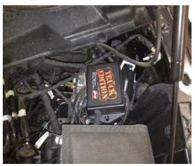
**13)** The switch can be routed through the firewall or can be left in the engine compartment next to the module. Connect the switch as shown.
