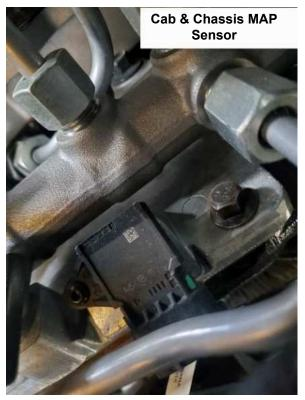
**9)** Plug the stock MAP sensor connector into the female MAP sensor connector on the Ag Diesel Solutions harness.
