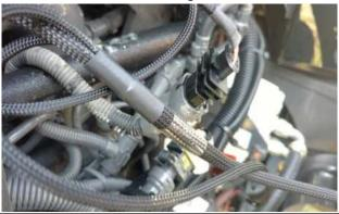
**4)** Locate the factory Injector Connector on the side of the cylinder head.
