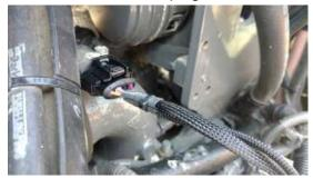
**3)** Insert the male MAP sensor connector from Ag Diesel Solutions module into the MAP sensor on the intake. Connect the factory male MAP sensor connector from the engine into the female connector on the Ag Diesel Solutions module harness.
