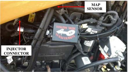
**2)** Locate the factory MAP Sensor connector on the intake manifold and unplug.
