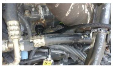
**5)** Insert the male injector connector from the Ag Diesel Solutions Module harness into the female injector connector on the cylinder head. Insert the female connector from the Ag Diesel Solutions module harness into the male injector connector on the engine
