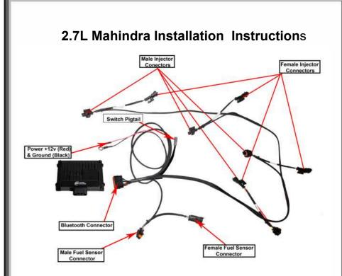
**1)** On the drivers side, under the hood, locate the fuel sensor connector and the 4 injector connectors
