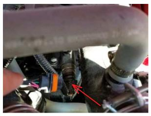
**3)** Looking directly over the top of the engine locate and unplug the 4 individual injector connectors.You will want to start at the back of the engine (firewall side) with injector connector "A" and work your way toward the engine fan ending with injector connector "D".
