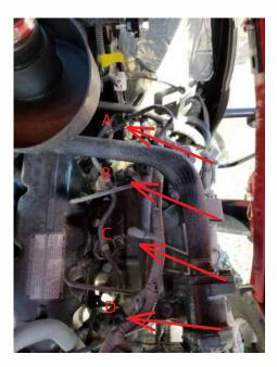
**4)** Plug the Ag Diesel Solutions male connector into the female stock injector. Plug the male stock connector into the Ag Diesel Solutions harness.
