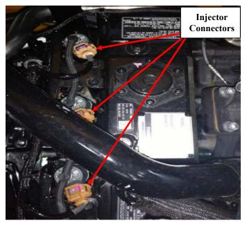
**2)** Unplug all four of the stock injector connectors. Press and hold the release tab on the connectors and gently pull the connectors
