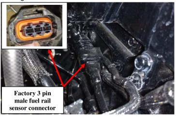
**7)** Insert the 3-Pin male connector from the module harness into fuel rail sensor. Make sure the connector latch is on the ramp side of the sensor.
