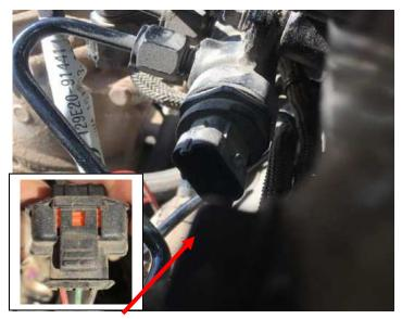
**8)** Connect the Factory 3-Pin male connector from the engine harness to the female 3-Pin Connector on the Ag Diesel Solutions module harness.
