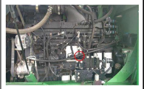
2) Use a 4mm allen wrench to disconnect the stock ECM Engine Connector 2
