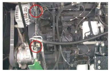
**5)** Plug the harness into the module. Mount the module with supplied zip ties away from any excessive heat or moving parts. Note: Zip tie the module to the factory wire harness. Mounting the module with the switch connector down will help prevent moisture from collecting into the module connector.
