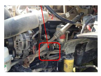
Disconnect the stock ECM Harness by pushing the Locking Lever down to release. Remove the harness from the ECM.
