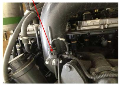
6) Disconnect the stock MAP sensor and plug Male connector from module into the stock MAP sensor. Plug the Female connector from the module into the stock MAP sensor wiring harness.
