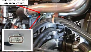
**4)** On the Ag Diesel Solutions module harness, the gray 10 pin female injector connector will now plug into the factory male injector connector that was unplugged from the valve cover in Step 2.
