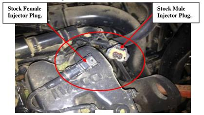
3) Route the Module Harness as shown in the pictures below. The Module Case will be located closer to the Fan side of the engine.
