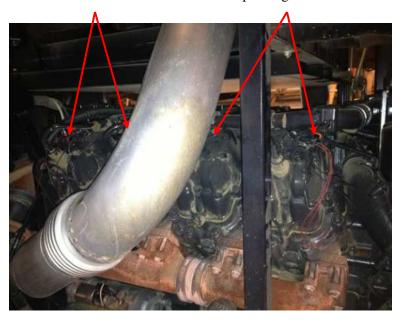
2) Disconnect all 8 sets of stock Injector Plugs. Press the Release Tab on the connector and gently pull the connector apart.
