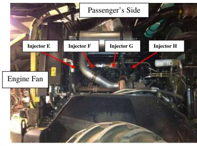
4) Connect all 8 sets of Injector Plugs from the Module harness into the stock injector plugs.
