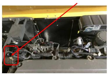
5) Disconnect the stock Exhaust Pressure Sensor.
