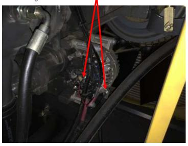
9) Mount the module with the connector on the bottom side, as to reduce the chance of moisture from getting into the module harness. Keep away from excessive heat and moving parts.
