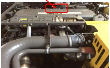
2) Disconnect the stock female Injector Harness plug located on the Bottom. Connect the female plug from the Performance Module Harness into the male Injector Harness Plug. Connect the stock female Injector plug into the corresponding male Harness plug on the new Harness. \*Note: Use the Injector Connector on the Performance Module Harness marked "Bottom". The connectors on the module harness are Black that connect to the bottom plug.
