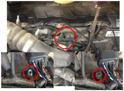
2) Plug the male connector from the module into the stock female connector on the engine. Plug the stock injector harness that was removed in Step 1, to the female connector from the module.
