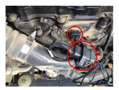
**3)** Locate the MAP Sensor. It is on the same side of the engine as the air intake and it will be closer to the "Fan side" of the engine.
