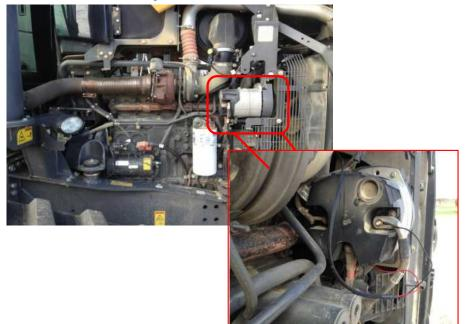
7) Plug the Harness into the module. Mount the module with supplied zip ties away from any excessive heat or moving parts. Note: Zip tie the module to the factory wire harness. Mounting the module with the connector down will help prevent moisture from collecting into the module connector.
