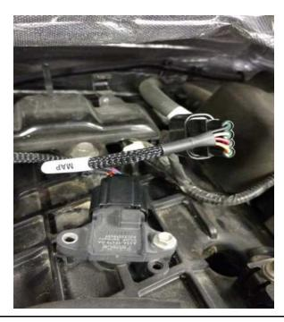
**5**) Disconnect the Factory Female T-MAP Sensor connector from the T-MAP Sensor.
