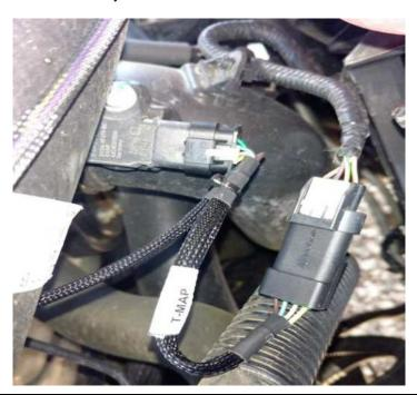
7) Remove the bypass plug from the Ag Diesel Solutions harness, and plug the harness into the module.
