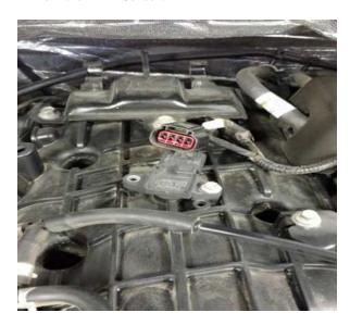
**4)** Utilize the portion of the ADS harness labeled MAP. Connect the ADS Female connector to the MAP Sensor. Then connect the ADS Male connector to the Factory Female MAP Sensor connector.
