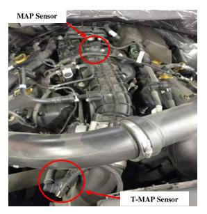
**3)** Disconnect the Factory Female MAP Sensor connector from the MAP Sensor.
