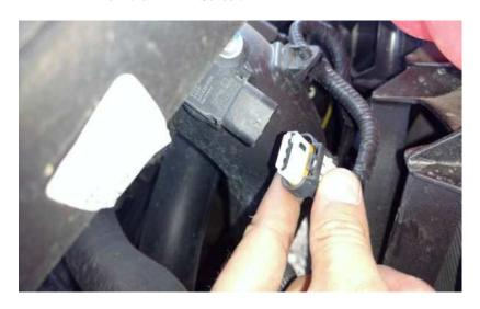
**6)** Utilize the portion of the ADS harness labeled T-MAP. Connect the ADS Female connector to the T-MAP Sensor. Then connect the ADS Male connector to the Factory Female T-MAP Sensor connector.
