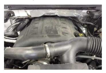
2) With the cover removed, locate the MAP & T-MAP Sensors. The MAP Sensor can be found on top of the intake manifold. The T-MAP Sensor can be found near the throttle body inlet.
