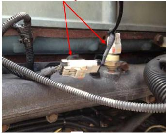
5) Route the power and ground wires to the alternator located on the passenger's side of the engine. Connect the red wire to +12 volts and the black wire to ground.
