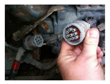
3) Plug Female Connector from module into the stock Mack Male harness
