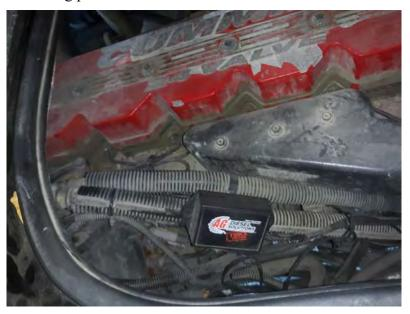
8) Once you have installed the module, connect the switch to the switch pigtail. Once connected you can zip tie it to the module and leave it in place.
