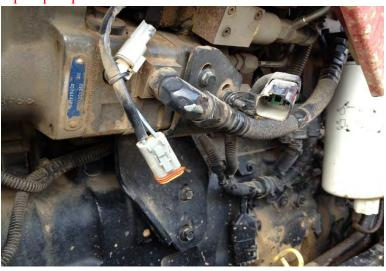
**3)** Connect the female injection control valve connector from the Ag Diesel Solutions harness into the stock male connector.
