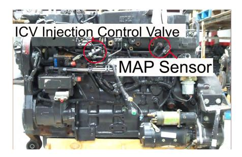
2) Connect the male injection control valve connector from the module into the stock female connector.
