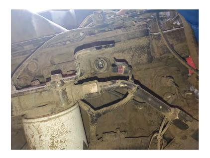
**5**) Connect the Female MAP sensor connector from the Ag Diesel Solutions harness into the stock male MAP sensor connector.
