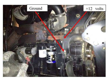
7) Mount the module in a safe location using the supplied wire ties. Secure the module away from any excessive heat and moving parts.
