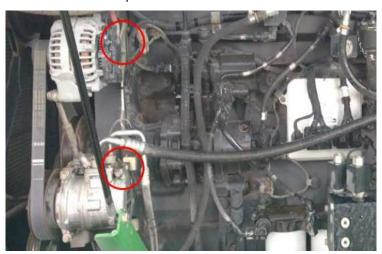
**5)** Plug the harness into the module. Mount the module with supplied zip ties away from any excessive heat or moving parts. Note: Zip tie the module to the factory wire harness. Mounting the module with the switch connector down will help prevent moisture from collecting into the module connector.
