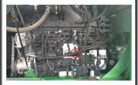
2) Use a 4mm allen wrench to disconnect the stock **ECM Engine** Connector 2
