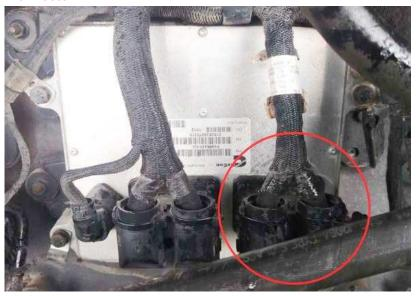
**3)** Plug the female connector from the Ag Diesel Solutions harness to the male connector of the stock harness. The 4mm bolt will need to be tightened to secure the connectors. Then, connect the Ag Diesel Solutions male connector into the stock female connector located on the ECM Engine Connector 2.
