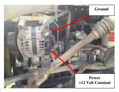
6) Connect the module connector to the module. Use the supplied wire ties to mount the module with the wiring connector horizontal (as shown) or mount vertical with the connector on the bottom side (to avoid collecting moisture). Keep away from any excessive heat sources.
