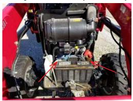
**6)** Mount the module with the connector on the bottom side, as to reduce the chance of moisture from getting into the module harness. Keep away from excessive heat and moving parts. Note: Zip tie onto the factory computer wire harness works well. Mounting the module as shown will help prevent moisture from collecting into the module connector.
