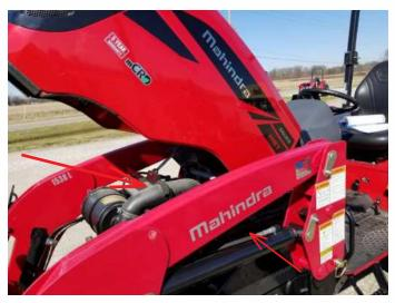
**2)**The fuel sensor connector is a 3 pin connector located on the driver side of the engine at the end of the fuel rail. Press the release tab on top of the connector, and pull it straight out. Plug the Ag Diesel Solutions male connector into the female stock connector. Plug the male stock connector into the Ag Diesel Solutions harness.
