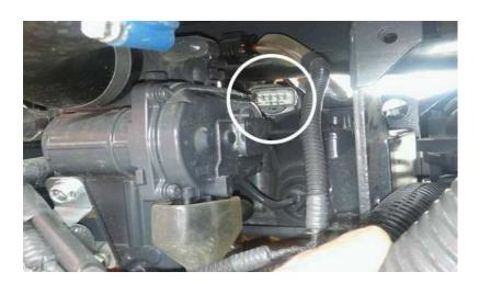
**2)** Unplug the stock injector connector. Press and hold the release tab on the connector and gently pull the connector apart.
