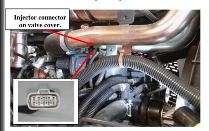
**4)** On the Ag Diesel Solutions module harness, the gray 10 pin female injector connector will now plug into the factory male injector connector that was unplugged from the valve cover in Step 2.
