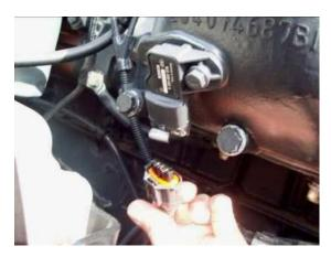
8) Connect the black wire with ring terminal to a good chassis
