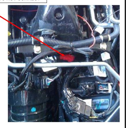
**9)** Connect red wire with ring terminal to a 12V constant source The left wire of intake air heater relay is good (Also alternator works).
