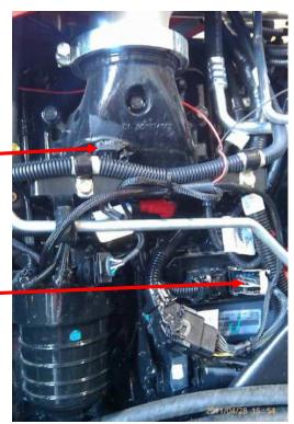
**3)** Plug the male connector from the module into the 16-pin ECM port.
