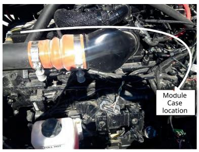
**4)**On the Ag Diesel Solutions harness, the female injector connector located closest to the Module Case will connect to the Male Injector Plug wiring located closest to the Flywheel-side of the engine.
