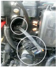
**9)**Connect red wire with ring terminal to a +12V constant source. Connect the black wire with ring terminal to a good chassis ground.
