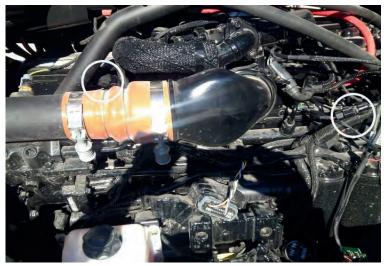
**2)**Unplug both sets of stock injector connectors. Press the release tab on the connector and gently pull the connector apart.
