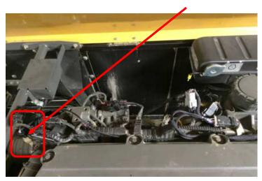
5) Disconnect the stock Exhaust Pressure Sensor.
