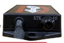
STK - Stock Mode - 0% HP Increase Position 2 - Up to 15% HP Increase HI - High Mode - Up to 30% HP Increase
