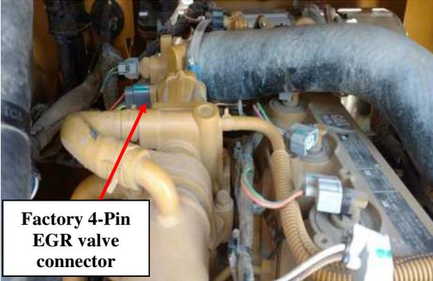
6) Remove the factory male injector connector located on the engine harness from the EGR Valve. Press and release the locking tab to disconnect.
