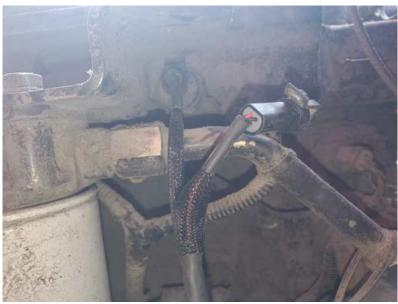
5) Connect the red wire with a ring terminal to a constant 12 volt source. Connect the black wire with a ring terminal to a good chassis ground. Wiring can be routed over the engine to the Alternator.
