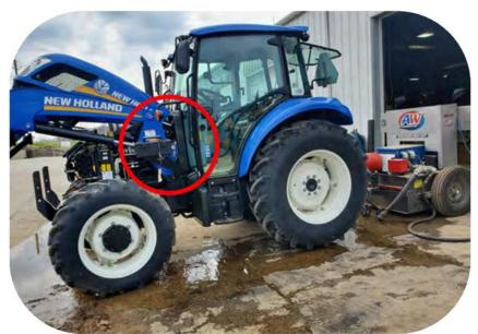
**Step 1)** Locate the fuel system on the engine. If you are looking forward through the cab, it will typically be on the left hand side of the engine. You will see the common rail with the injector lines coming out of it. Orientation may vary based on the model of equipment.
