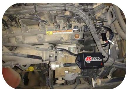
Step 4) Mount the module with the connector on the bottom side, as to reduce the chance of moisture from getting into the module harness. Keep away from excessive heat and moving parts.
