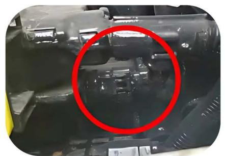
**Step 2)** Locate the fuel pressure sensor. It can be located at either end of the common rail or protruding outward in the middle of the rail. This is a 3-Pin connector.
