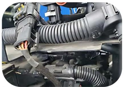
**Step 3)** Connect the 3-Pin male fuel pressure connector on the Ag Diesel Solutions Module to the stock 3-Pin female connector on the engine. Then connect the stock 3-Pin male connector on the engine harness to the 3-pin female connector on the Ag Diesel Solutions module Harness.
