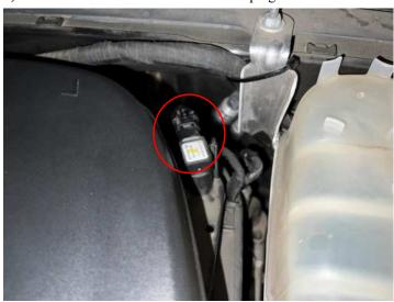
**4)** Plug the Female module MAP connector into the vehicle MAP sensor.
