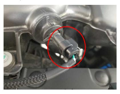
**8)** Plug the Male module IAT connector to the vehicle harness Female IAT sensor connector.
