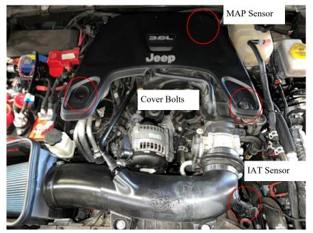
3) Locate MAP sensor connector and unplug from MAP sensor.
