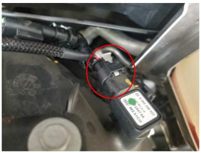
**5)** Plug the Male module MAP connector to the vehicle harness Female MAP sensor connector.
