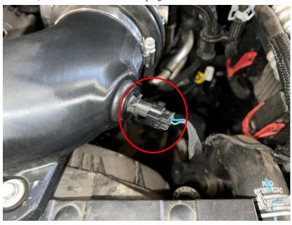
7) Plug Female module IAT connector into vehicle IAT sensor.
