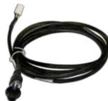
Module switch can be ran inside the cab for easy performance adjustment. Module switch can be secured in engine bay if desired. Module will default to HIGH setting if switch is not connected
