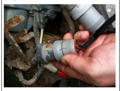
**4)** Plug Male Module Connector into the stock Female Mack harness.
