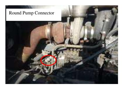
2) Unplug round engine connector as seen in picture
