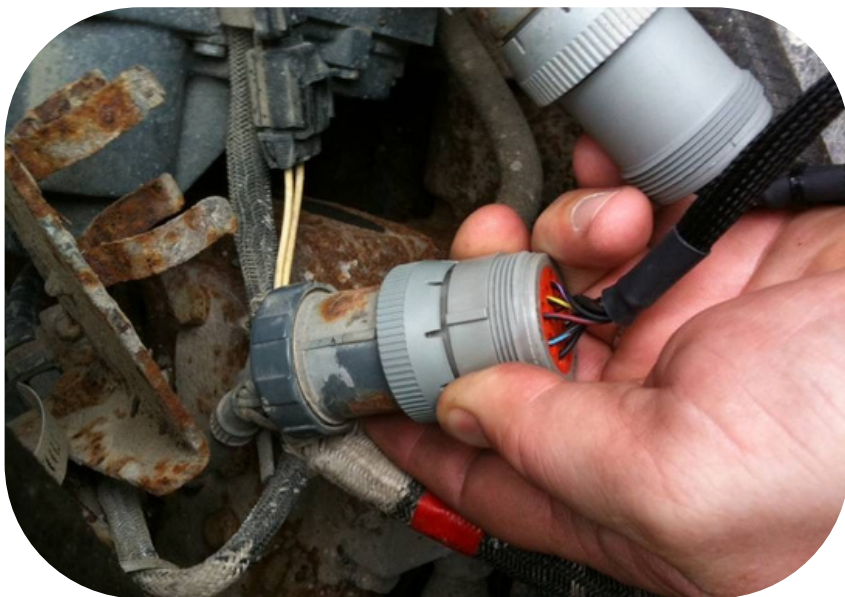
Step 3) Plug Female Connector from module into the stock Mack Male harness
