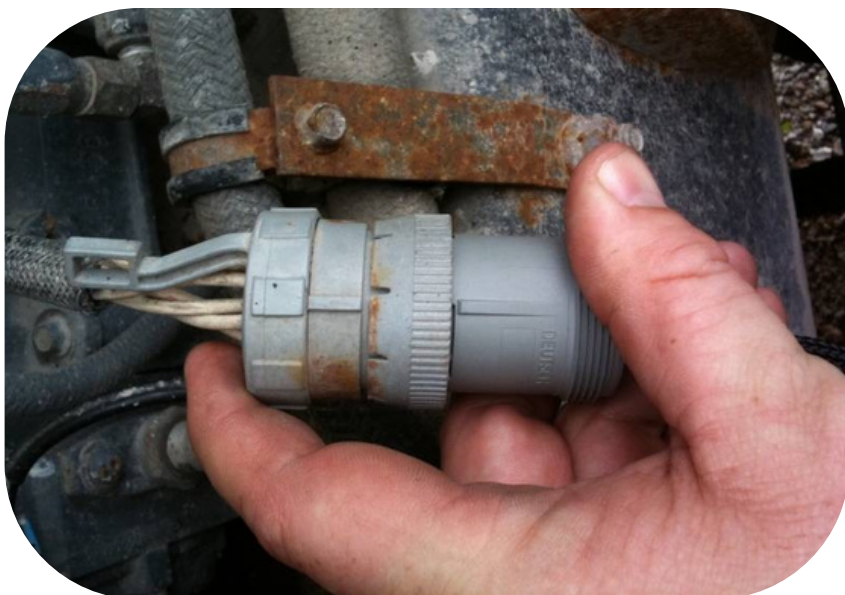
Step 4) Plug Male Module Connector into the stock Female Mack harness.
