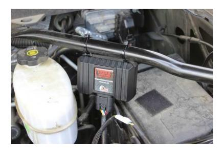
**10)** Once you have installed the module, connect the switch to the switch pigtail. Once connected you can zip tie it to the module and leave it in place.
