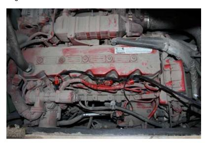
**4)** Locate the first injector connector near the flywheel side of the engine. Plug the female injector connector on the Ag Diesel Solutions module harness labeled "flywheel" into the stock male injector connector. The male injector connector on the Ag Diesel Solutions module harness will plug into the female injector connector.
