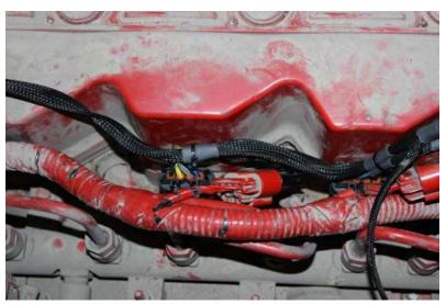
**5)** Continue to the next 2 sets of injector connectors. Repeat Step 4 to connect each pair of injector connectors. Note: The Ag Diesel Solutions harness will connect in series between the stock injector plugs and stock wiring plugs. All plugs on the new harness will be connected.
