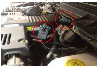
5) Plug both of the Ag Diesel Solutions injector connectors into the injector connectors on the engine. Do this for BOTH the front and rear injector connectors.
