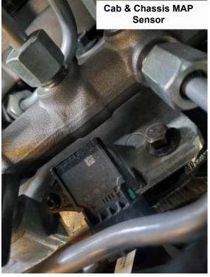
**9)** Plug the stock MAP sensor connector into the female MAP sensor connector on the Ag Diesel Solutions harness.
