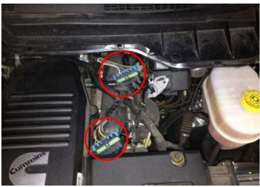
**4)** Plug the stock male injector connectors removed in Step 3 to the female connectors on the Ag Diesel Solutions module. Do this for BOTH the front and rear injector connectors.
