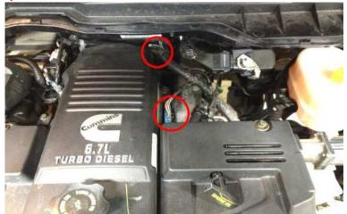
**2)** Unplug the engine connector labeled below. This will allow access to the rear injector connector.
