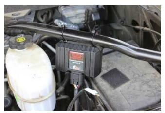
**13)** The switch can be routed through the firewall or can be left in the engine compartment next to the module. Connect the switch as shown.
