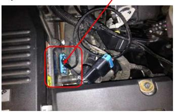
6) Plug the stock engine connector that was unplugged in Step 2.
