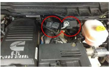
**3)** Unplug both the front and rear stock male injector connectors on the engine
