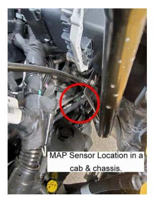
**8)** Unplug the MAP sensor and plug in the male connector from the Ag Diesel Solutions module into the MAP sensor.
