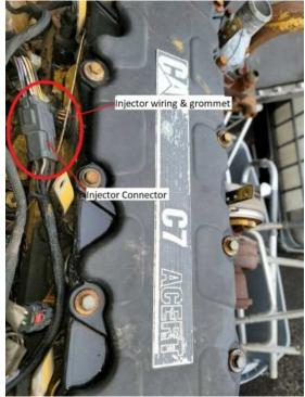
On some of the older CAT engines, injector plug might me located vertically mounted on side of engine as shown in diagram.
